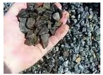
Figure 1. EAF steel slag aggregate. (from en.wikipedia.org/wiki/Construction)
